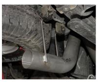
CONNECT TURNOUT #D EXIT PIPE TO THE REAR OVERAXLE PIPE. ROLL TURNOUT PIPE UNTIL YOU HAVE IT AT THE CORRECT ANGLE FOR YOUR TRUCK AND CONNECT WITH CLAMP #F. BUT DO NOT TIGHTEN.
