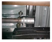
UNCLAMP EXHAUST IN FRONT OF STOCK MUFFLER. IF YOU HAVE AN EXTENSION PIPE BETWEEN THE CONVERTER AND MUFFLER- DO NOT REMOVE! LEAVE ALL RUBBER GROMMETS IN PLACE. INSTALL HANGERS AS PROVIDED. INSTALL HEADPIPE #A ONTO YOUR EXISTING STOCK FRONT PIPE AND CONNECT WITH CLAMP #G. USE JACKSTAND TO SUPPORT THE CONVERTER.
